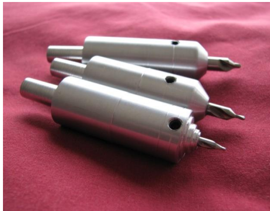
Project example – engineering topics: inexpensive chucks for center drills.
