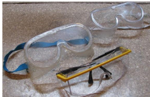
Fig. 4.1: Safety glasses. Use versions with ANSI Z87 label. ANSI is short for American National Standards Institute. Chemistry goggles, as also shown here, are not recommended for metal work, since they may block the vision too much
