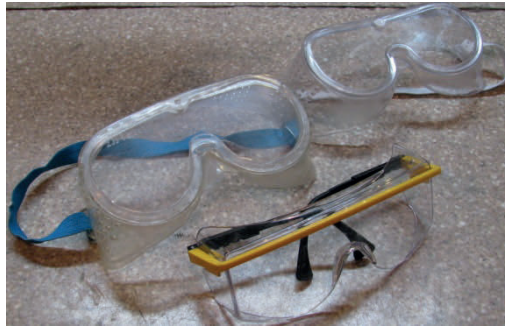
Fig. 2.1: Safety glasses. Use versions with ANSI Z87 label. ASNI is short for American National Standards Institute. Chemistry goggles, as also shown here, are not recommended for metal work, since they may block the vision too much
