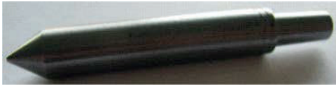
Fig. 5: Morse #0 taper (for Sherline) as extensions of the tailstock spindle cut from SAE 4140. See vol. 1 for details about how to cut a Morse taper, or perhaps get the LatheCity angle protractor (Morse taper/arbor cutter)
