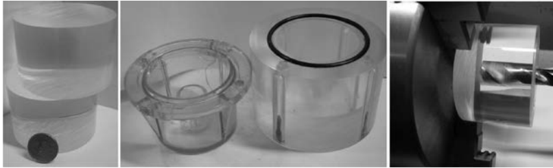
Fig. 4: Left) Machining a 2" acrylic solid round; Center) Here to replace a broken oil cup of a vacuum turbo pump; Right) SIEG lathe
