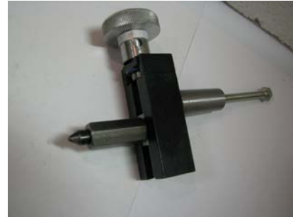
A MT0 center can be mounted using the MT0 arbor mount
