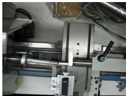
Taper turning with a drive dog. Try this out with an aluminum round. See latheCity vol. 1t
