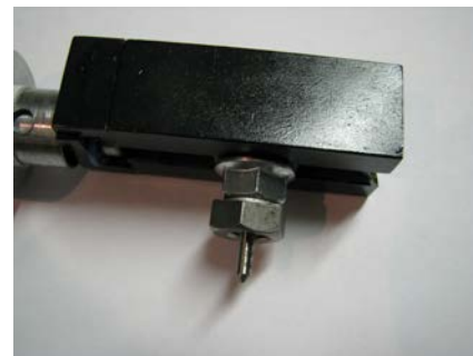
Use a second nut to protect the threads of the saddle.
