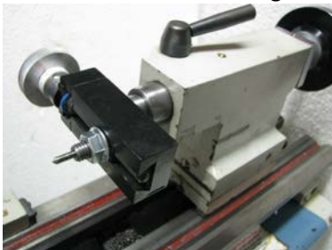
Tool mounted in tailstock of a lathe
