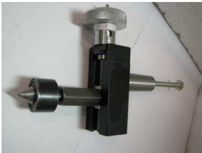
A small life center can be mounted using the MT0 arbor mount
