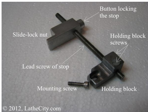
Fig. 1: Assembling the compound slide lock.
