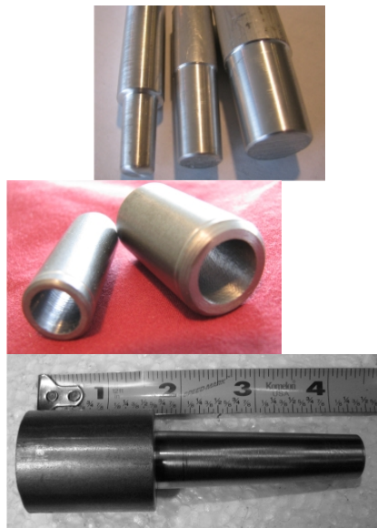
Fig.: Left) MT0, MT1, MT2 taper (reduced length), Middle) MT0 and MT1 arbors, right) full length MT2. LatheCity sells these type of accessories.
