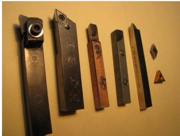
Fig. 2: Different types of (right hand) lathe cutting tools. From left to right: ceramic inserted tip cutter, carbide inserted tip cutter, two brazed carbide cutters, and HSS cutting tool. All from Sherline, except the blue brazed carbide cutter (on the right) which is from Harbor Fright Tools. Shown also are two inserts. The diamond shaped one with two cutting edges is from Sherline ($10 in 2011). The triangular shaped one with three cutting edges was purchased from MSC industrial supply ($5.59 in 2011). The grade of the inserts is unknown to me. Vol. 4 (milling operations) discusses how to make holder for inserted tip cutters since purchasing less expensive inserts of various shapes and sizes requires having a variety of tool holders on hand. This quickly becomes quite pricy and it is not too hard making those tool holders with a small mill (see vol. 4)
