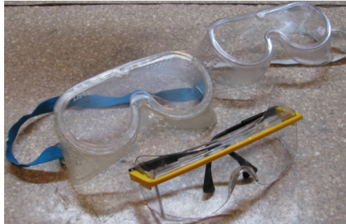
Fig. 1: Safety glasses. Use versions with ANSI Z87 label. ANSI is short for American National Standards Institute. Chemistry goggles, as also shown here, are not recommended for metal work, since they may block the vision too much
