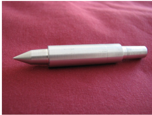
Fig. 2: Morse #0 taper as extensions of the tailstock spindle cut from SAE 4140. See vol. 1 for details about how to cut a Morse taper, or perhaps get the LatheCity angle protractor (Morse taper/arbor cutter)
