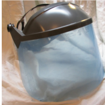
Fig. 2: Full face shield with plastic foil that needs to be peeled off
