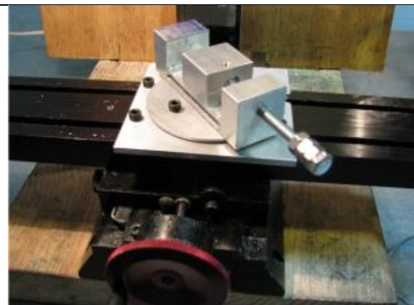
Swiveled base for the self-made vise – working with a rotary table
