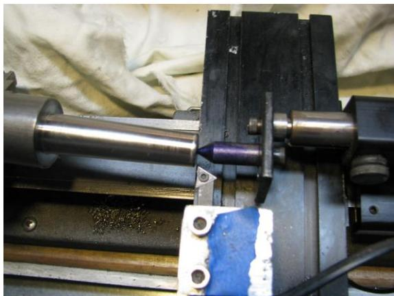
**Typical application:** Accessory for benchtop / tabletop lathes. Adapter mounts in a Morse #0 arbor, e.g., in the tailstock spindle of a small tabletop lathe and connects to a dead center (pin).
