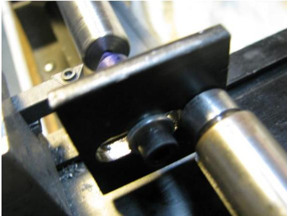
Slide the dead center along the keyway until it aligns with the center hole of your work piece. Tighten the two bolts of the adjustable dead center.
