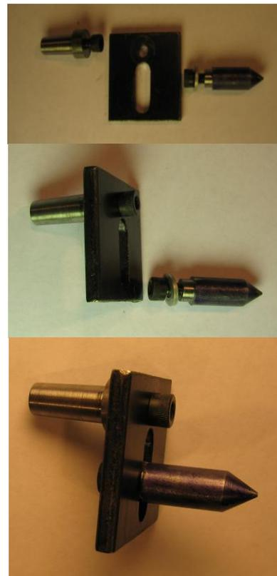
**Assembling the tool.** To save on shipping costs, this tool is shipped disassembled. For mounting it, two screws need to be tightened, see images.
