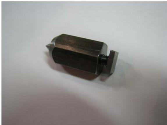
**Size and details** The bearings we use have an outer diameter (O.D.) of only 5/16" and an inner shaft diameter of 1/8". A 1/4" O.D. tool steel pin (60° included angle) is pressed in the bearings. The bearing is pressed in a hex shaped steel arbor that is
